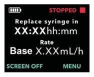
b. After pressing OK, the Pump automatically exits Initial Setup and displays the Status Screen in stopped mode.
