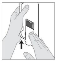
7. Slide the Battery Cover onto the Pump (see *Figure D*).
