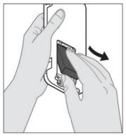
b. Remove the Battery (see Figure F).
